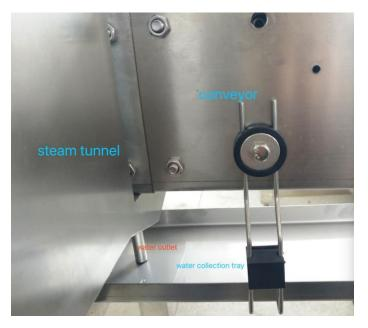
The HF-1500M steam shrink sleeve tunnel was designed and developed by HOWFOND company as a result of rapid growth in the use of shrink sleeves, particularly in the form of Sleeve Labels, which highlighted the need for low to high speed shrinking systems to match the performance of sleeve application machines such as the HF-250M, sleeve labeling machine.
